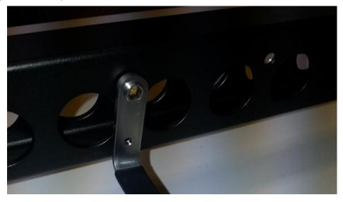
4. Install the belt guard with the cutout for the load bar using two screws removed during step 1
