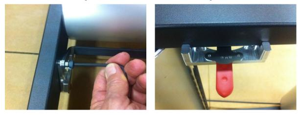
6. Assembly is complete and should look like that shown below. The load bar in this picture is furthest away from the middle drum and in the no load position. To add load, gently pull the handle inboard and move it forward to swing the load bar closer to the
