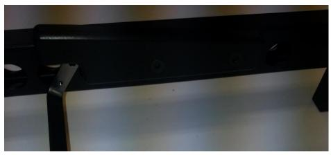
5. Insert the shoulder bolt into the pivoting mechanism of the load adjustor and insert the bolt into the forward screw hole on the frame rail. The bottom of the adjustment mechanism has two tabs which abut against the bottom of the rail as shown below. Tighten the shoulder bolt until it is snug.
