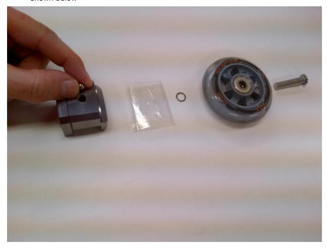
**3.** Place the shim on top of the hole on the bumper body as shown below.
