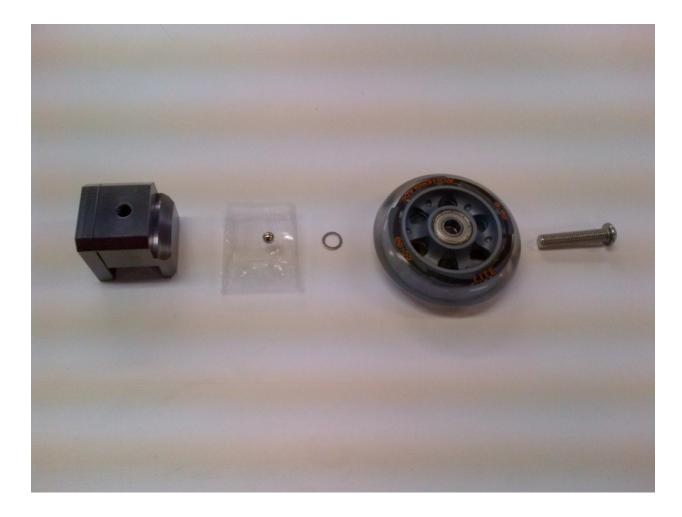
2. Insert the ball bearing into the threaded hole on the top of the bumper body as shown below
