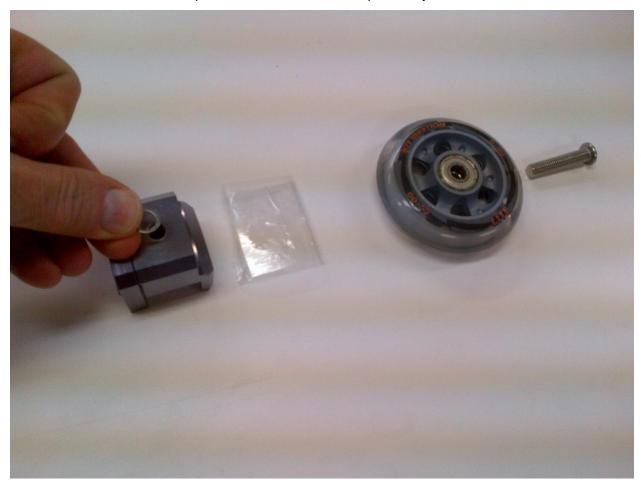
**4.** Place the screw through the roller wheel and insert it into the threaded hole. Make sure the shim fits over the screw..
