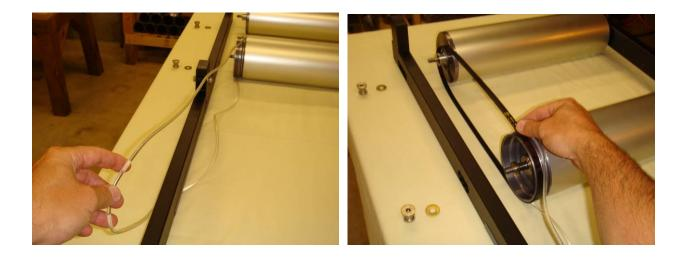
11. Below to the left is the proper configuration of the belts prior to installing the remaining frame rail. Install the frame rail onto the shafts with the round shoulders. The shoulders are sized to fit into slots on the inboard side of the rail. Below to the right is a photo of the rail installed on the shafts ready for washer and clamp nut installation.
