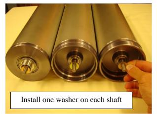
3. Pair a washer with the square hole with the shafts with square shoulders and install one washer on each shaft as shown below. Failure to use the high strength square washers will result in damage to the rails.
