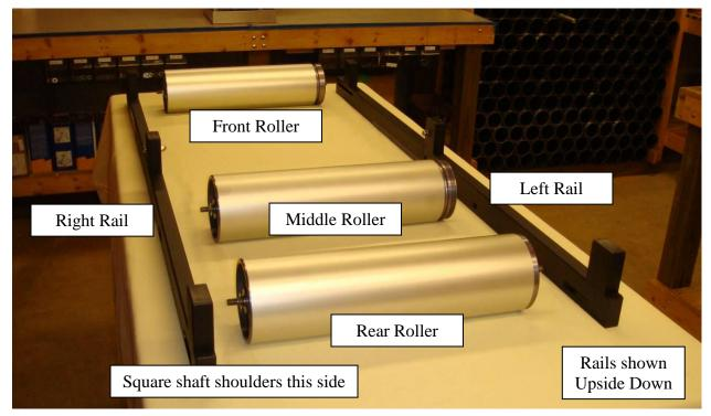
5. Mount the frame rail onto the shafts with the square shoulder. The square shaft shoulders are designed to prevent rotation of the shaft and fit into slots on the inboard side of the rails. You will have to rotate the shafts to align the shoulders with the slots. The rail must mate with all three shafts and a round hole washer and shaft clamp nut are needed on each roller shaft. Do not install the washers or nuts until proper engagement of the shafts is obtained.
