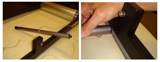
**15.** Pick up the rollers and turn them over so that they are standing on the rail legs to allow belt installation and tensioning.
