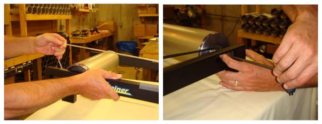
**17.** (*Skip the following, if you are assembling Travelers*) Install the flywheel belt guard in the position shown using three hex screws provided using a 4 mm hex wrench. The photo below shows a left side installation.
