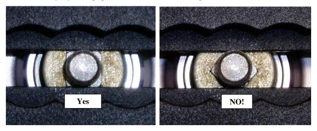
7. Install a washer with a round hole on the front roller shaft. Then install the shaft clamp nut and position the roller in the slot appropriate for your bike's wheelbase. Recommended wheel positioning data can be found in the TruTrainer User's Manual. Secure the nut with a 6 mm hex wrench.
