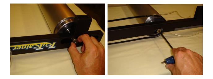
**13.** Install a washer and a shaft clamp nut on the rear roller, but do not tighten it. This nut needs to remain loose to allow the flywheel drive belt to be tensioned.
