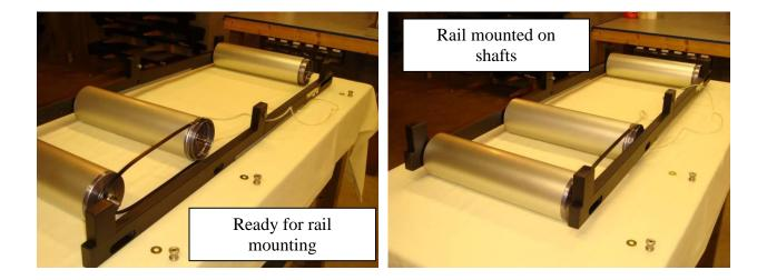
**12.** Install washers and clamp nuts on the front and middle rollers and secure both shafts with a 6 mm wrench.
