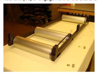
8. Before installing the washers or tightening the shaft nuts, verify that the flats on the end of the shafts are engaged in the slots in the rails. Failure to obtain proper engagement will result in damage to the rails.
