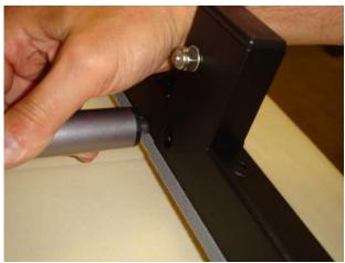
**16.** Pick up the rollers and turn them over so that they are standing on the rail legs to allow belt installation and tensioning.
