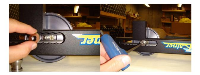
**14.** Install a washer with a round hole on the rear roller shaft. Then install the shaft clamp nut, but do not tighten this nut. It should be loose to allow the tension of the flywheel drive belt to be adjusted. You are now ready to begin installation of the drive belts.
