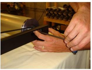
**18.** (Skip the following, if you are assembling Travelers) Install the flywheel belt guard in the position shown with two hex screws using a 4 mm hex wrench. An older design used three screws; the latest belt guards feature a cutout for an optional load bar and only requires two bolts. The photo below shows a left side installation.
