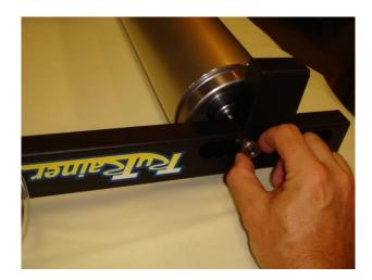
**10.** Install a washer on the middle roller shaft and install a shaft clamp nut. Secure the nut with a 6 mm hex wrench
