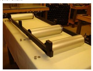
**13.** Install washers and clamp nuts on the front and middle rollers and secure both shafts with a 6 mm wrench.
