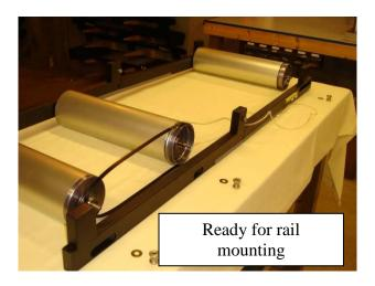
7. Mount the frame rail onto the shafts with the square shoulder (drive side). The square shaft shoulders are designed to prevent rotation of the shaft and fit into slots on the inboard side of the rails. You will have to rotate the shafts to align the shoulders with the slots. The rail must mate with all three shafts and a round hole washer and shaft clamp nut are needed on each roller shaft. Do not install the washers or nuts until proper engagement of the shafts is obtained.
