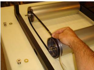
**6.** Below to the left is the proper configuration of the belts prior to installing the remaining frame rail. Install the frame rail onto the shafts with the round shoulders. The shoulders are sized to fit into slots on the inboard side of the rail. Below to the right is a photo of the rail installed on the shafts ready for washer and clamp nut installation.
