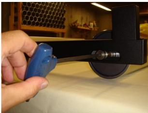
**15.** Insert the telescoping end of the carrying handle into the hole provided on the inboard side of the middle frame leg. Collapse the handle and insert the fixed end into the hole on the opposite rail. When the frame is extended, the handle prevents the rails from folding. The rollers can now be safely repositioned.
